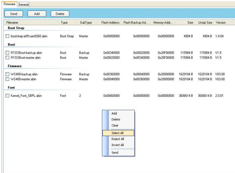
8. Click **Send** to send the firmware files to your printer. During the transmission, LED 1 blinks green. In the **Download Firmware** dialog box, the message shows the file your printer is downloading, and the progress bar indicates the progress of downloading.
