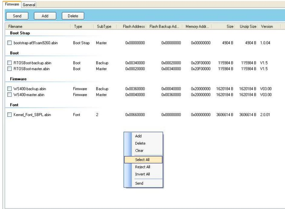
9. Click **Send** to send the firmware files to your printer. During the transmission, LED 1 blinks green. In the **Download Firmware** dialog box, the message shows the file your printer is downloading, and the progress bar indicates the progress of downloading.
