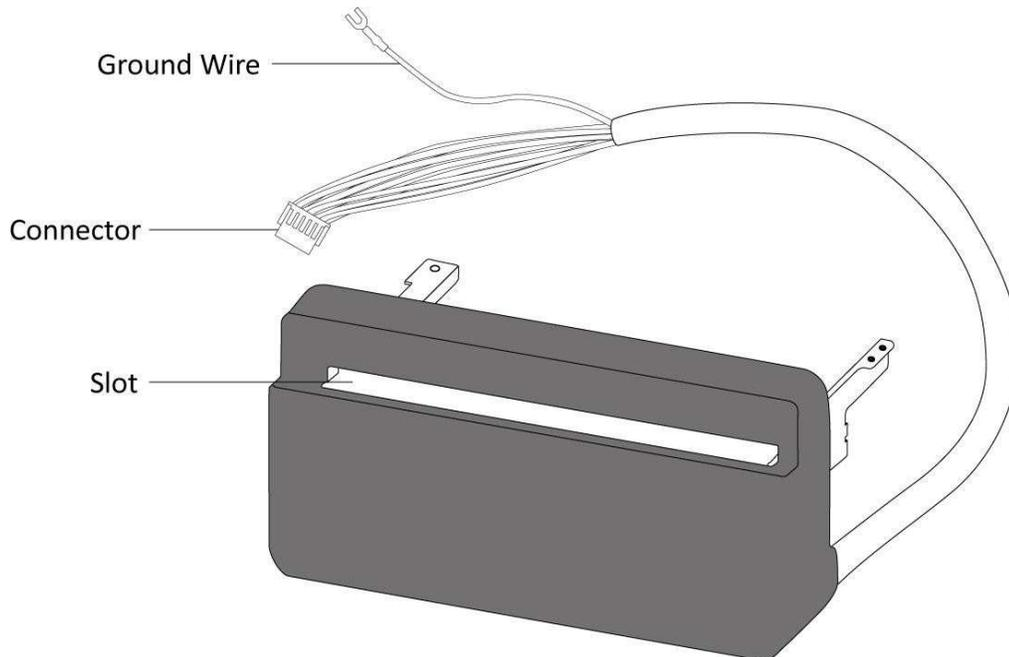
A cutter is used to cut the label after it is printed out. Full cutter cuts a label off from a media roll.
