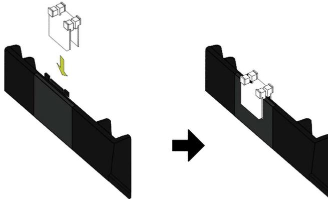
8. Attach the antenna to the **Antenna** port. The figures below show the correct (left) and incorrect (right) wiring.
