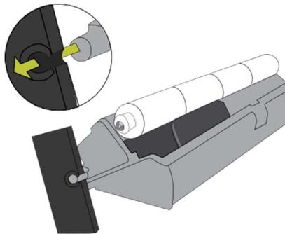
3. Use a coin to tighten the thumbscrew to the hole beside the right dowel.
