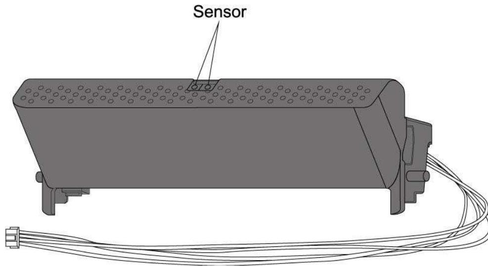
A dispenser automatically removes the liner from the printed label. The dispenser sensor detects if a peeled label is taken away.
