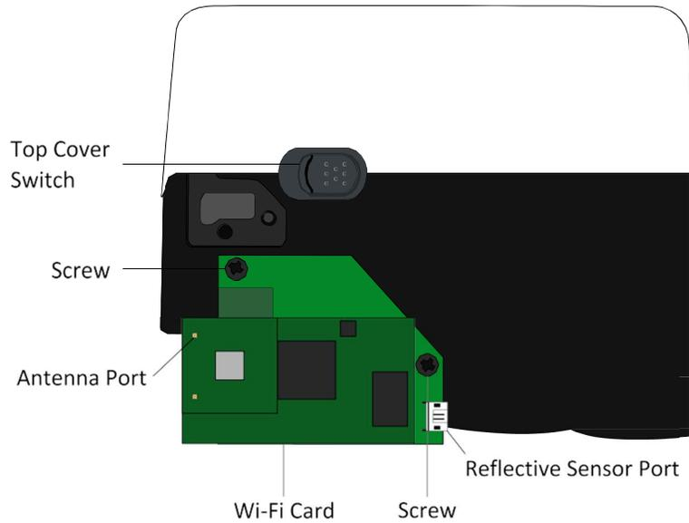
3. On the right side of your printer, find two screw holes under the top cover switch, align the two holes on the Wireless LAN card with them and secure the card with two screws.
