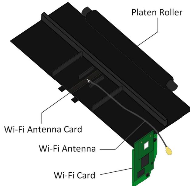
6. Paste the foam pad to the surface behind the Wireless LAN antenna card.
