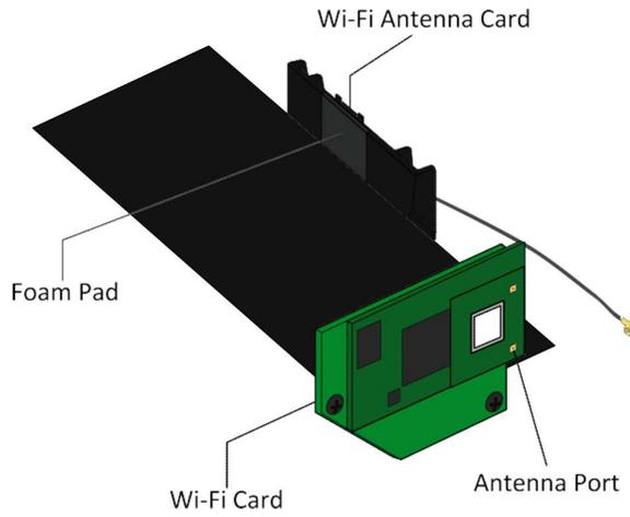
7. Use the clip to fasten the Wireless LAN antenna card and the foam pad.
