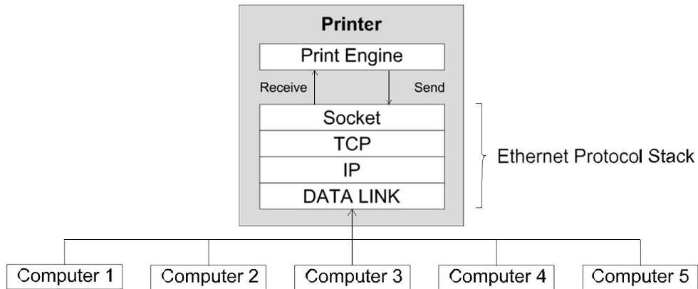
As the figure shows, the network architecture includes several layers, and each layer corresponds to the layer in the Open Systems Interconnection (OSI) model.
