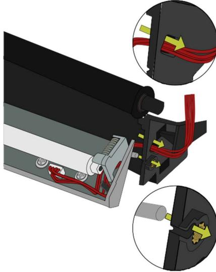
2. On the left side, gently press the dispenser to the right to give some space for the left dowel and slightly push the left dowel into the hole.
